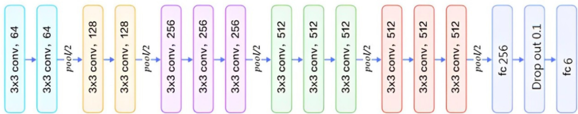
Figure 7 VGG16 architecture. This figure illustrates the VGG16 architecture with additional modifications. It includes the incorporation of a fully connected layer with 256 units, a dropout rate of 0.1 to mitigate over-fitting, and an output layer with 6 units. These changes are made to enhance the model’s performance in classifying temporomandibular joint disorders (TMJD) stages.
