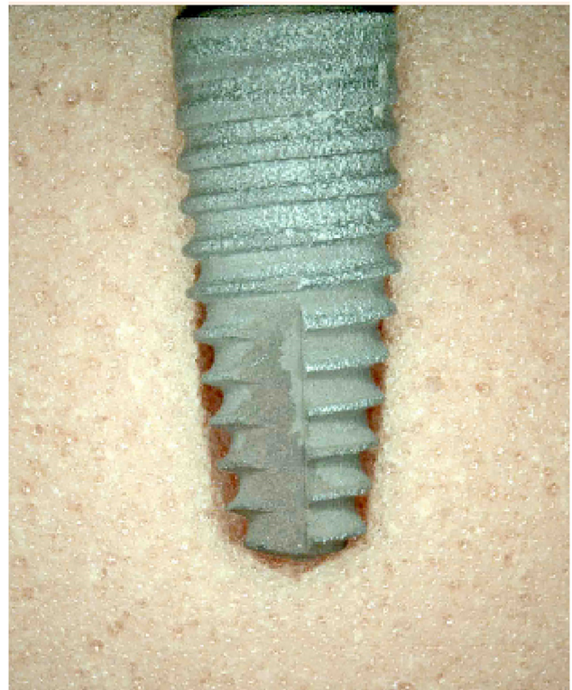
Figure 8 Microscopic observations of BLT implant insertion. Cutting chamber of implant BLT, which is approximately 5 mm in length, does not engage with the implant socket. BLT: Bone level tapered.
